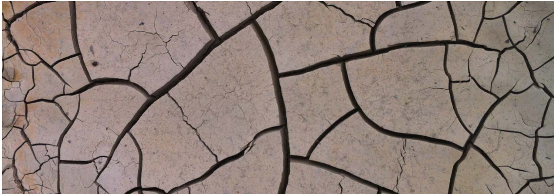
Figure 8: Clays form a wide group of minerals of a very fine grain size (<4 microns). Determining their mineralogy is of great importance to understand soil behavior (e.g. swelling clays)
